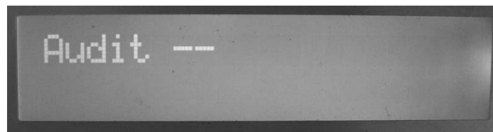
Figure 24 – Display in Service Mode; showing the first sub-menu - Audit
