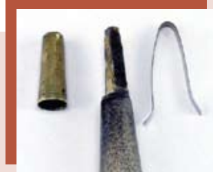
Detail of trimming tool with ferrule removed and watch-spring cutter formed to desired contour.
