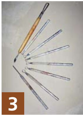
3 Carving tools from bottom to top: needle tool, several sizes and various shaped loop tools, curved blade of a clean up tool.
