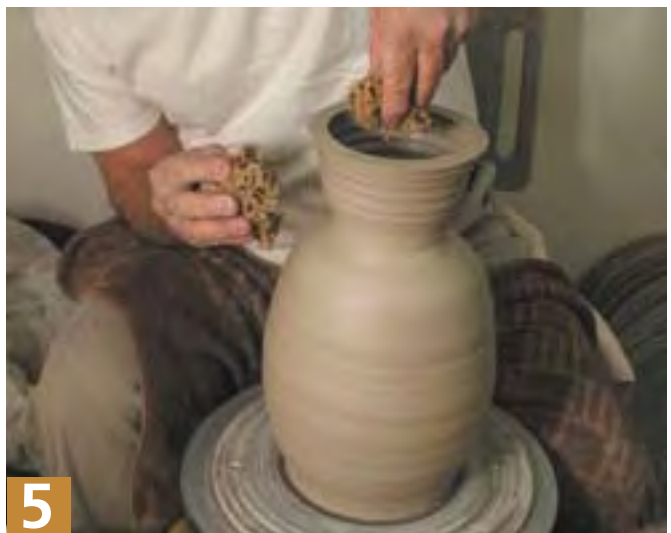
5 Turn the wheel slowly and use your fingers to attach the top to the body, then smooth the joint (bottom). Dry to leather hard. Place upside down on a bat and trim the bottom to match the bowl-shaped interior.
