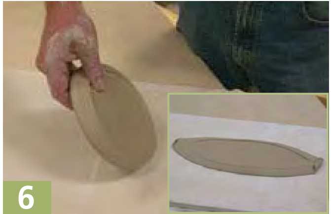
6 Immediately remove the disc from the wheel and stretch it into an oval by throwing it onto a canvas surface. Make sure the piece hits the table at an angle so the disc stretches. The clay should make a "wisp" sound instead of a "WHAM!" when it hits the table.
