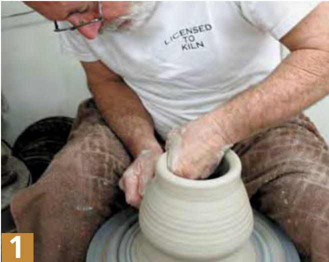
1 Form body: Throw a 4-pound ball of clay into a bulbous shape about 9 inches tall. Measure the opening with calipers. Set aside until leather hard.
