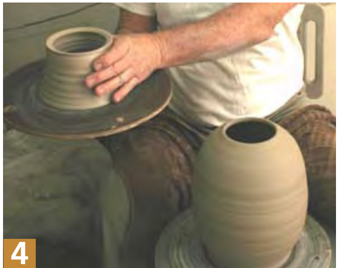
4 Attach top and body: With its bat still attached, place the body on the wheel head. Score and slip the rim. Turn the top piece upside down and place onto the body.
