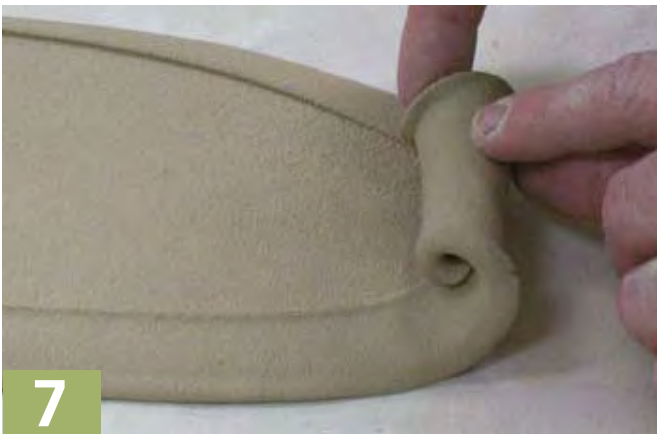
7 After stretching the disc, roll the edges over to eliminate any sharpness. This also creates a relationship between the curled area and the handles that will be attached later.
